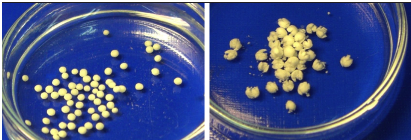
Fig. 3: Disintegration of classical MCC pellets (Avicel PH 102) and MCC Sanaq Burst pellets with a drug load of 80% (w/w) Chloramphenicol after staying 5 sec in water (study sponsored by Pharmatrans Sanaq [10]).
